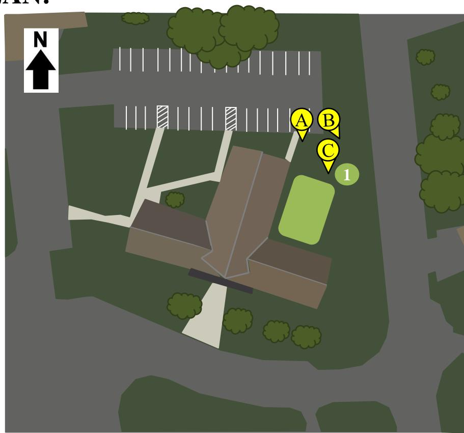
**BIORETENTION SYSTEMS:** A bioretention system can be installed in the turf grass on the northeast side of the church to capture, treat, and infiltrate runoff from the roof. The bioretention system can reduce sediment and nutrient loading to the local waterways and increase groundwater recharge. Building a bioretention system can also provide habitat for birds, butterflies, and pollinators.
